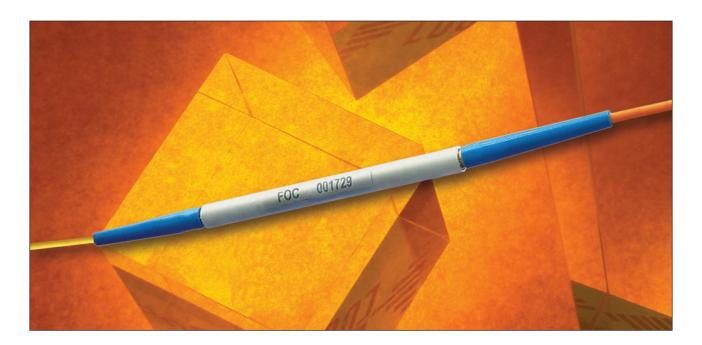
Mode conditioning cables are employed to prevent problems arising from the use of singlemode lasers for transmissions over multimode fibres. They induce higher modes thus limiting differential mode delay. This is done by injecting the singlemode laser systematically outside the centre of the MM fibre's core.
