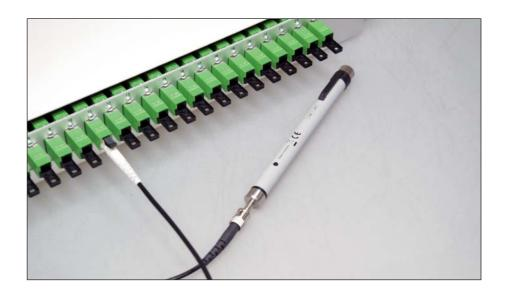
Wherever fiber breaks, microbendings or bad splices occure in fiber-optical links, the focussed laser light is scattered. These faults can be seen through the outer fiber cladding or the cable jacket.
